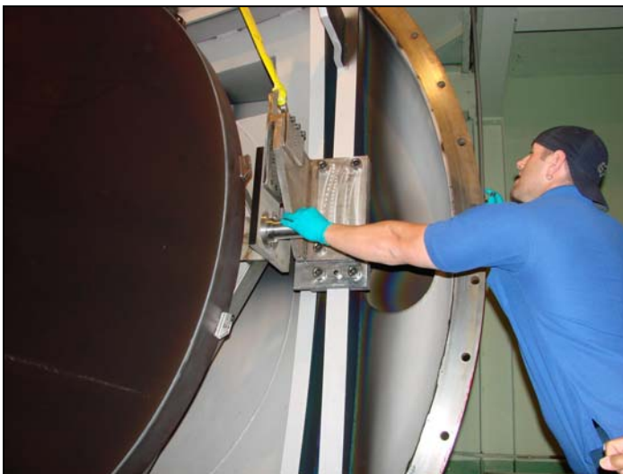
Load the optic into the tank
